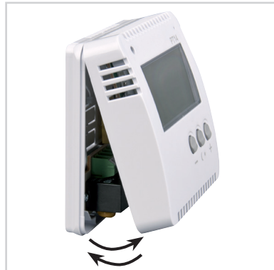
Fig.4 Place the part with the electronics on the bottom part and secure with a locking screw.
